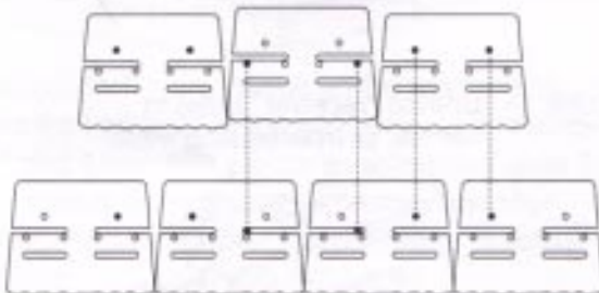
FIGURE 13 Inset wall Pinning on one-half bond
