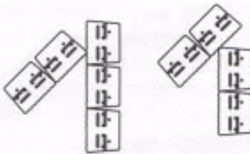
FIGURE 12 Low Angle Inside Corner
